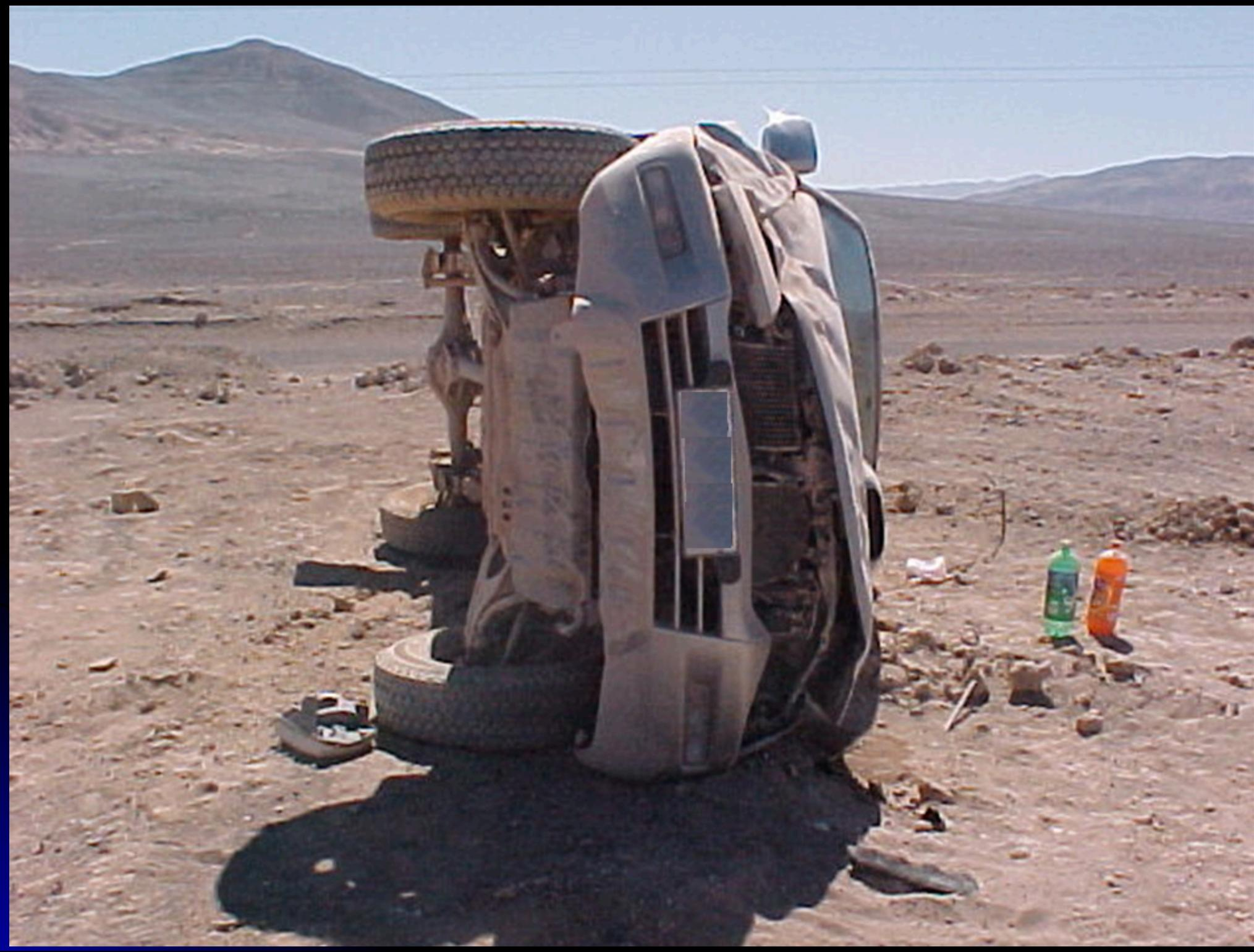
**ESTA IMAGEN MUESTRA QUE AL TENER SOLO UNA BARRA PROTECTORA EN LA PARTE TRASERA Y NO LLEVAR BARRA INTERNA, EL PILOTO Y COPILOTO, SUFREN EL MAYOR DAÑO.**
